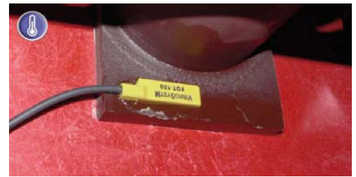
FOT - Fiber optic temperature sensor for monitoring end-windings, isophase bus bars, switchgears and circuit breakers
