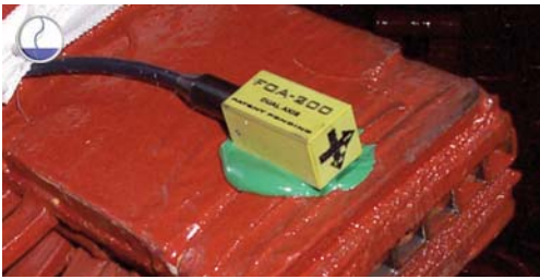
FOA - Fiber optic accelerometer for end-winding vibration monitoring
