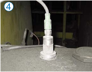
4 VSM797S - Piezoelectric accelerometer for stator core vibration monitoring
