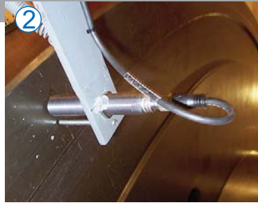
2 PES probe for axial thrust displacement
