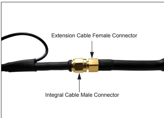
1. Make sure the integral cable's male connector is well secured to the extension cable's female connector.
