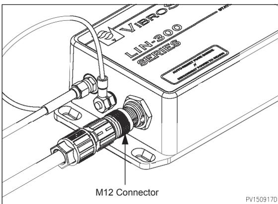
3. Make sure the M12 connector is firmly secured in place.
