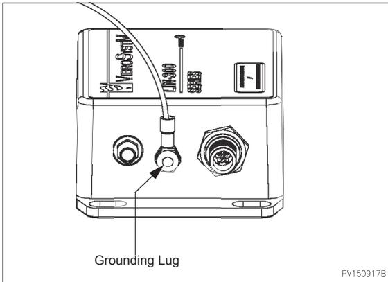
1. Make sure the grounding lug is firmly secured to the LIN-300's grounding terminal.
