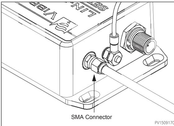
2. Make sure the integral cable's SMA connector is firmly secured to the LIN-300's SMA socket.
